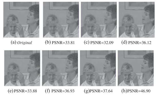
Fig. 10. Recovery performance for fully decomposable CS (FDCS) under various sampling rates. The overall sampling rates for the first and second rows are 0.25 and 0.45, respectively. (a): Original; (e): KCS; (b)(f): FDCS with r_t = 0.45 ; (c)(g): FDCS with r_t = 0.6 ; (d)(h): FDCS with r_t = 0.75 .
