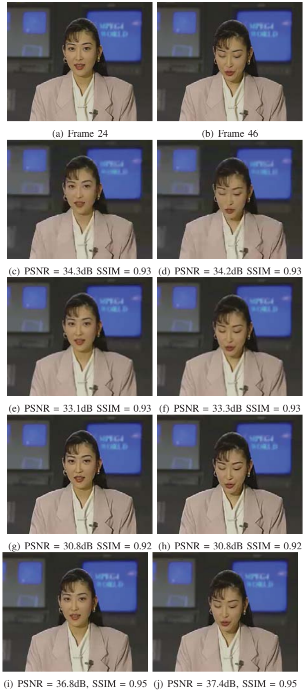
Fig. 7. (a) and (b) are the original frames from “Akiyo” sequence; (c) and (d) are standard-codec H.264/AVC frames; (e) and (f) are bicubic interpolated frames; (g) and (h) are LLE frames; (i) and (j) are the proposed video frames. Each example is compared under the same bit-rate = 240kbps.
