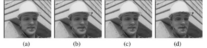
Fig. 11. Reliability mask for the second frame of Foreman sequence. The black dots denote unreliable pixels. (a) Warping result from the previous frame ( Q_s = 64 ). (b) Warping result from the next frame ( Q_s = 64 ). (c) Warping result from the previous frame ( Q_s = 32 ). (d) Warping result from the next frame ( Q_s = 32 ).
