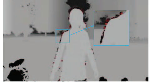
Fig. 3. The structure saliency, represented by the red points, of the temporally inconsistent region.
