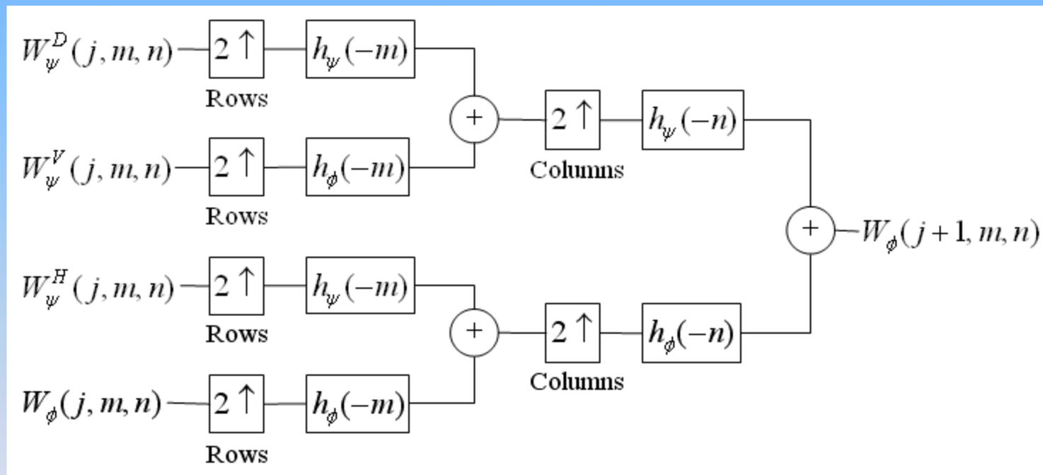
The two-dimensional FWT — the synthesis filter bank.
