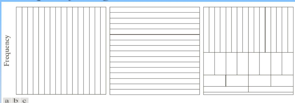
**FIGURE 7.23** Time-frequency tilings for the basis functions associated with (a) sampled data, (b) the FFT, and (c) the FWT. Note that the horizontal strips of equal height rectangles in (c) represent FWT scales.
