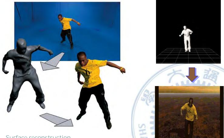
Surface reconstruction Using Visual-Hull and geometric constraints
